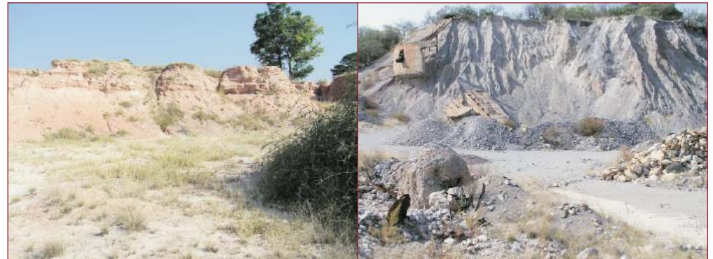
Figure 2. Tailings (slimes) dump (left) and waste rock dump (right) at Berg Aukas.
